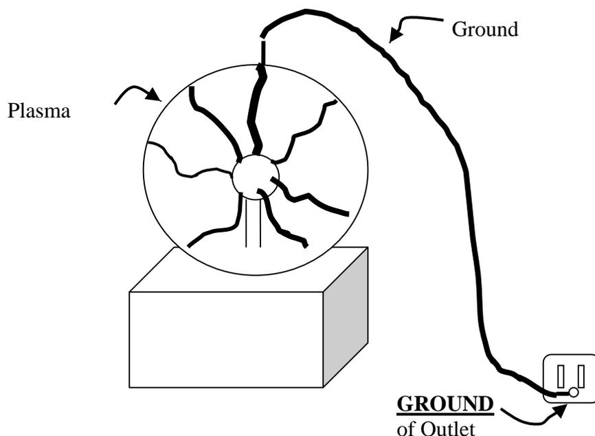
**Figure 1:** Ground wire used to hold a vertical streamer in place for examination of its spectrum
