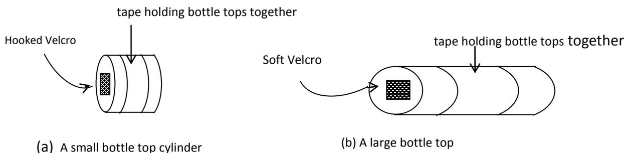
**Figure 1:** Bottle top cylinder details
