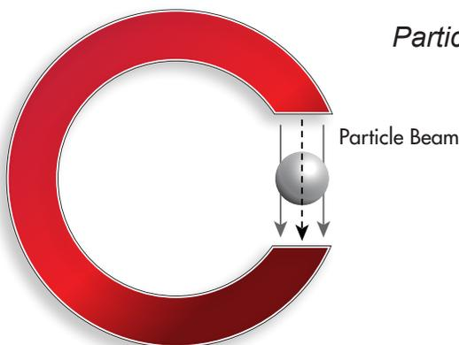
*Particle beam within the magnetic field of a C-shape magnet.*
