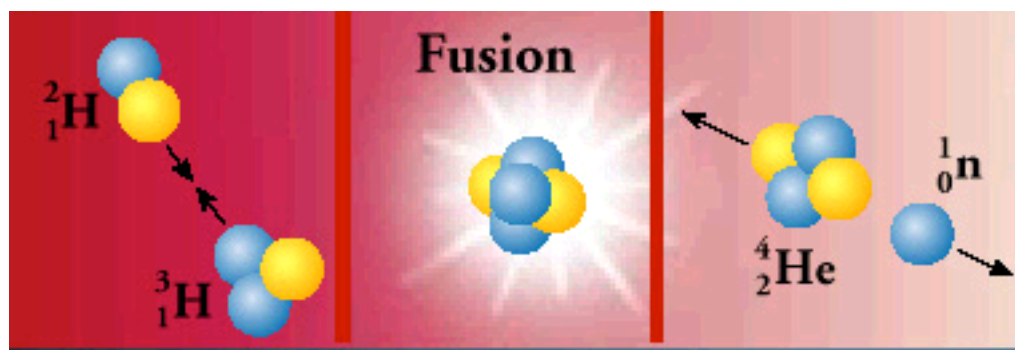
Fig. 14-3. A diagram showing a typical fusion reaction.
