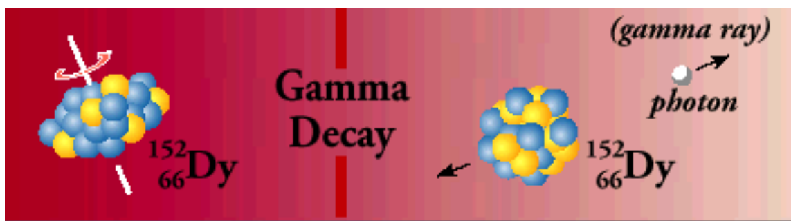
Fig. 3-6. A gamma ( \gamma ) decay.
